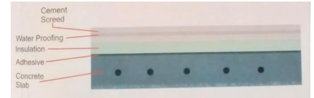
Roof over deck insulation
